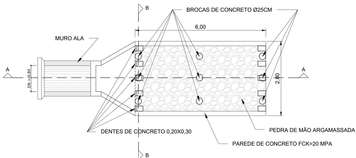
VISTA SUPERIOR - MURO ALA E DISSIPADOR SEM ESCALA
