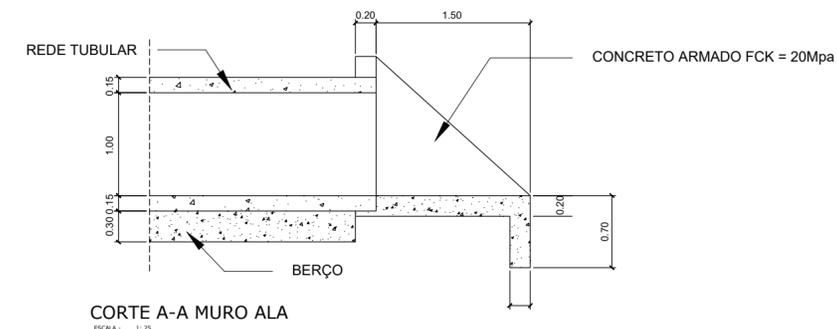
CORTE A-A MURO ALA ESCALA - 1:25
